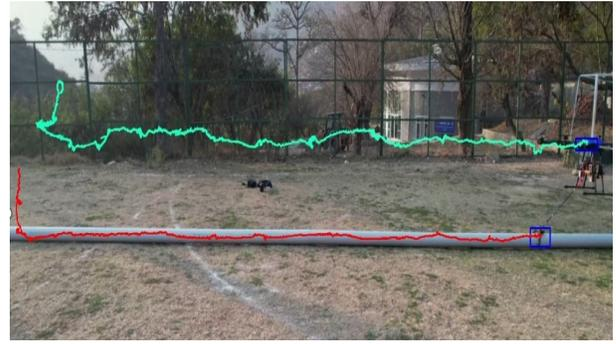
Fig. 12: Fully autonomous operation of aerial manipulator and end-effector trajectory.
